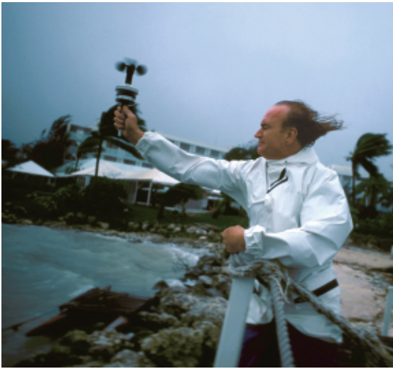
Figure 2 A meteorologist uses an anemometer during Hurricane Luis to measure wind speed.
