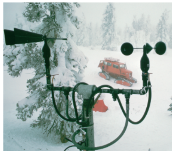
Figure 1 Weather instruments, such as these at Elk Mountain weather research facility in Wyoming, indicate wind speed and direction.
